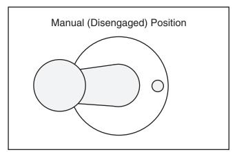
**Figure 35.** Downfeed selector in manual (disengaged) position.
